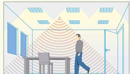
Maintained illuminance: Presence detected, with automatic dimming working in conjunction with daylight.
